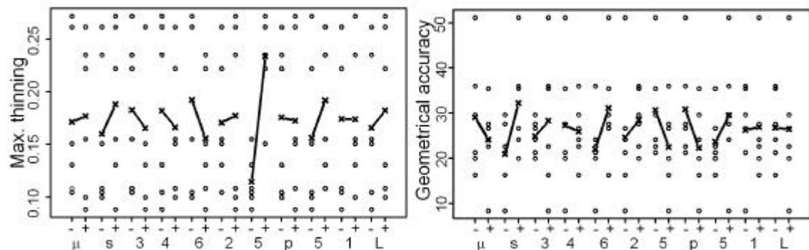
**Figure 5:** Main effect diagramme for two quality characteristics
