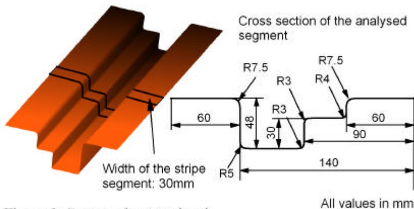
**Figure 1:** Design of a virtual rail
