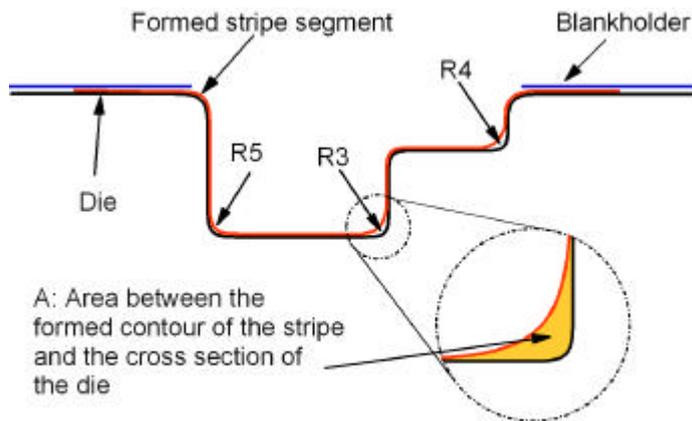
because there is only a virtual model which cannot directly be compared with a real structure. Therefore it is best to regard the outline of the die as the optimum to be fitted. The area between the formed blank and the die can be seen as a value, quantifying a loss of quality. **Figure 2** shows the described area. The thinning of the blank sheet can be regarded as a method to obtain a second value, giving further information on the forming result.
